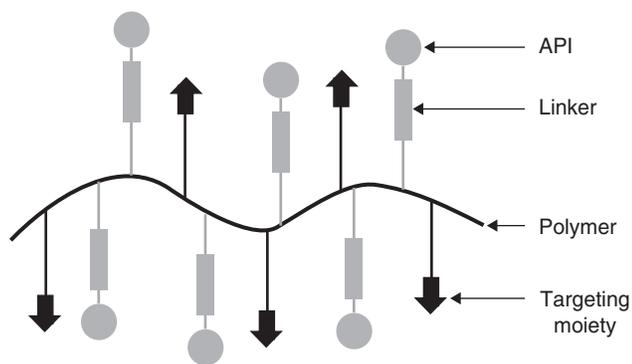
**Figure 1. Schematic representation of the Ringsdorf model of polymer therapeutics.** APIs, or drugs, and targeting moieties are attached to a polymer backbone. A single or several APIs and targeting moiety can be present on the polymer chain.
