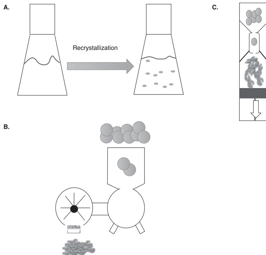
**Figure 1. Schematic of top-down and bottom-up nanocrystal production. (A)** Schematic of crystallization or bottom-up method of production. Top-down methods include **(B)** milling and **(C)** high pressure homogenization.
