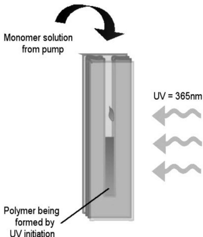
**Figure 2.** Schematic representation of the polymerization apparatus. A gradient of monomer solution was pumped into the polymerization apparatus while a constant ( $\approx 2.5$  mW) light source was used to polymerize the polymer.
